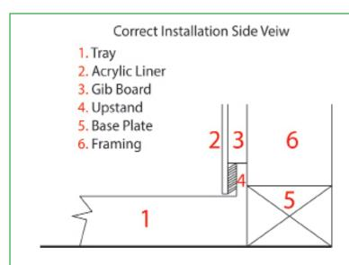
Pictured left, is a drawing depicting the correct installtion method of a tray in a standard GIB Board lined wall.
