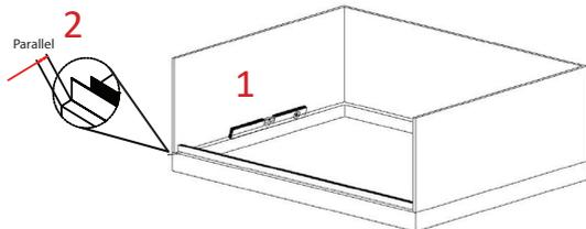
**Step 1** - Using a level, ensure the tray is level along all 4 edges prior to channel installation.
