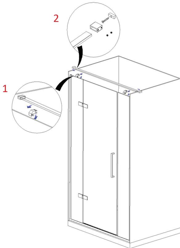
**Step 1** - Fit the retaining brackets to the top edge of the each glass panel. Their position along the edge of the panel is your choice, but they must be a minimum of 80mm from the wall linings to allow for the mounting block fitment.
