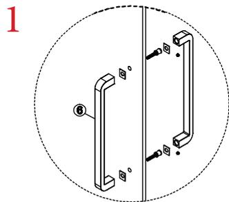
**Step 1-** Install the Handle onto the door panel.
