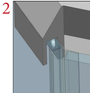
**Step 2-** Install the horizontal weatherseals. The rounded "bulb" shaped seal is installed onto the Hinged panels of glass. The concave seal is placed onto the trailing edge of the door panel.
