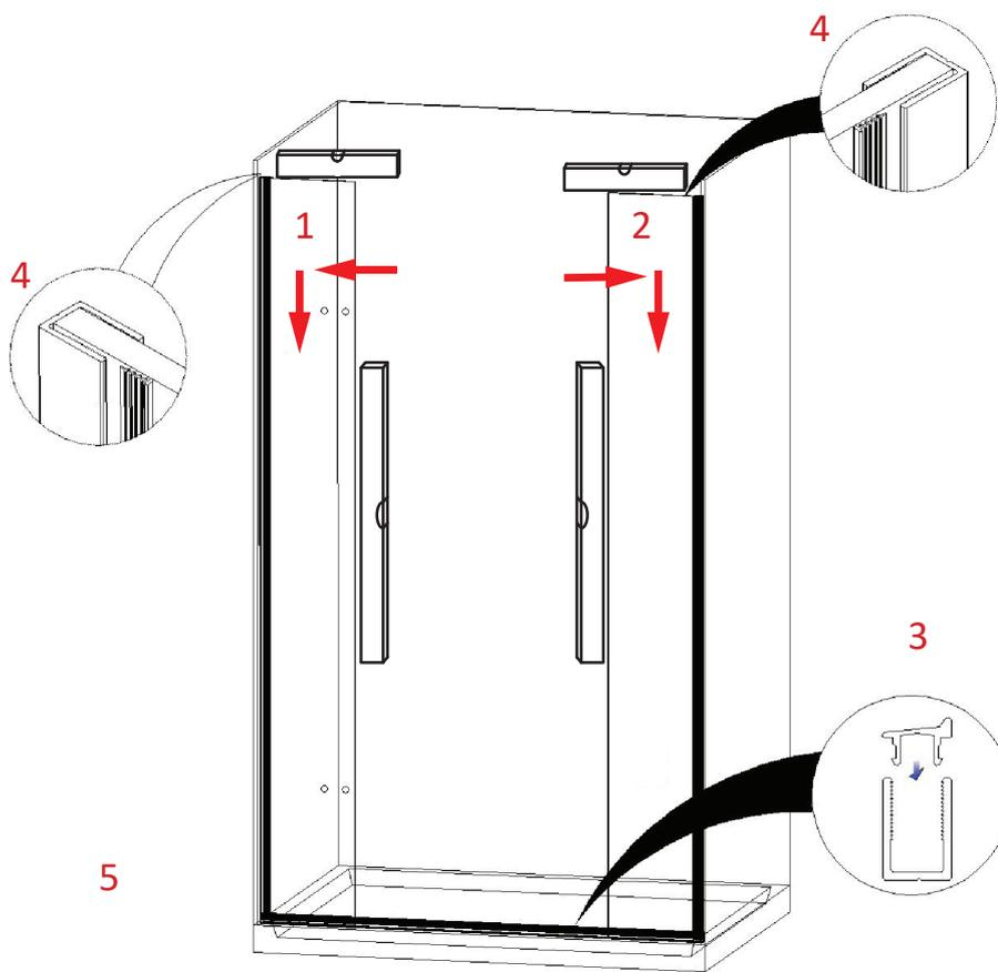
**Step 1** - Place the small glass hinged panel (with holes) into the wall and floor channel.
