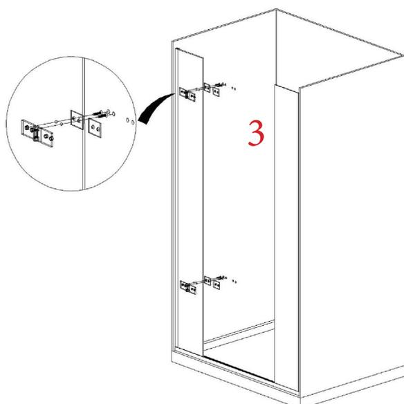
**Step 3-** Place blocks of either polystyrene, cardboard, or soft clothes onto the floor and place the door onto these carefully. You will need packers which are approx 115mm high.
