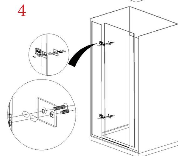
**Step 4 -** Offer the door up to the hinges and carefully thread the screws through the glass and onto the hinges. Tighten the screws up to a medium strength.
