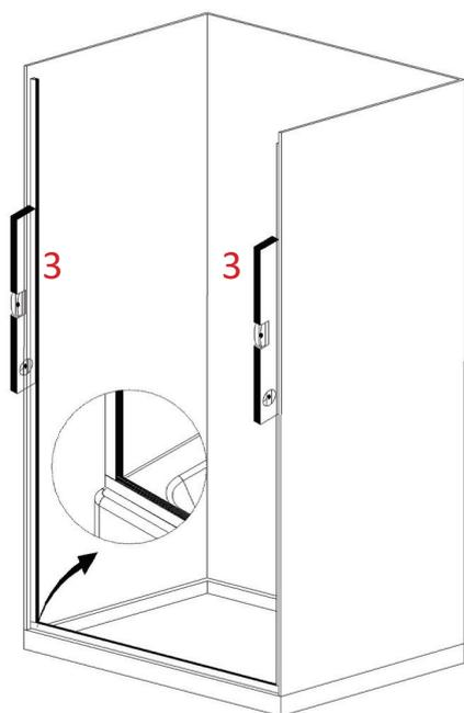
**Step 3**- Place the wall channel onto the top of the floor channel and align. Then using a level ensure the wall channel is vertically plumb, and mark the hole positions on the wall surface.
