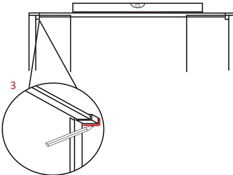
**Step 3** - Position the mounting blocks against the wall linings and mark their position by tracing the outline of the block onto the wall linings. Also check the support bar is level.
