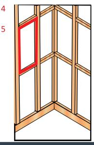
Step 4- Frame out the wall, or modify existing framing so that both sides, and the top and bottom of the Tile Niche are surrounded by framing.
