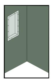
Step 8 - Cut the wall substrate to suit the outside dimension of the flange on the Tile Niche. Install the wall substrate.
