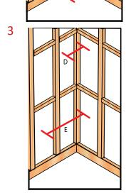
Step 3- Measure from the inside corner of the wall out to the preferred position of where the inner edge of the Tile Niche will be installed (D). Using a level mark this position on the adjacent studs and down to the bottom plate.
