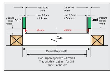
For example a 900x900x900 alcove tray after installation of 10mm wall boards on each side should have a wall to wall measurement of 880mm, top, middle and bottom ready to receive the wall liner which allows 875mm for the door to be installed.
