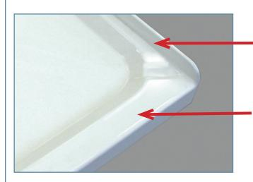
Here is the 40mm high Upstand which is installed hard against the timber framework of the wall. The GIB Board installs down to the top of this, and the Liner is installed over the Upstand and sealed to prevent water entering the walls
